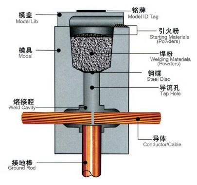
The EXOTHERMIC WELDING process is a method of making electrical connections of copper-to-copper or copper-to-steel in which no outside source of heat or power is required. In this process, conductors are prepared, placed in a purpose-designed graphite mold, and exothermically welded to produce a permanent electrical connection.
