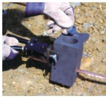
Step-06: Steel disk found inside the packaging box of welding material. Insert the steel disk (concave side up) into the mold. Hold the steel disk on the side of the mold and let it slide into place. Ensure that the steel disk is properly seated.
