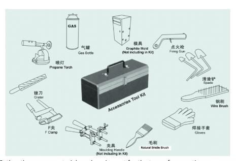
**STEP-01:** Gather the proper materials and equipment for the type of connection you are making. The typical EXOTHERMIC WELDING system requires, safety gloves a graphite mold, handle clamp, welding
