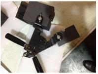
**Step-03:** Slide the handle clamp into the pre-drilled holes with the proper orientation for the thumbscrews. Tighten the clamp thumbscrews onto the mold. Close the grips to tightly lock the mold.
